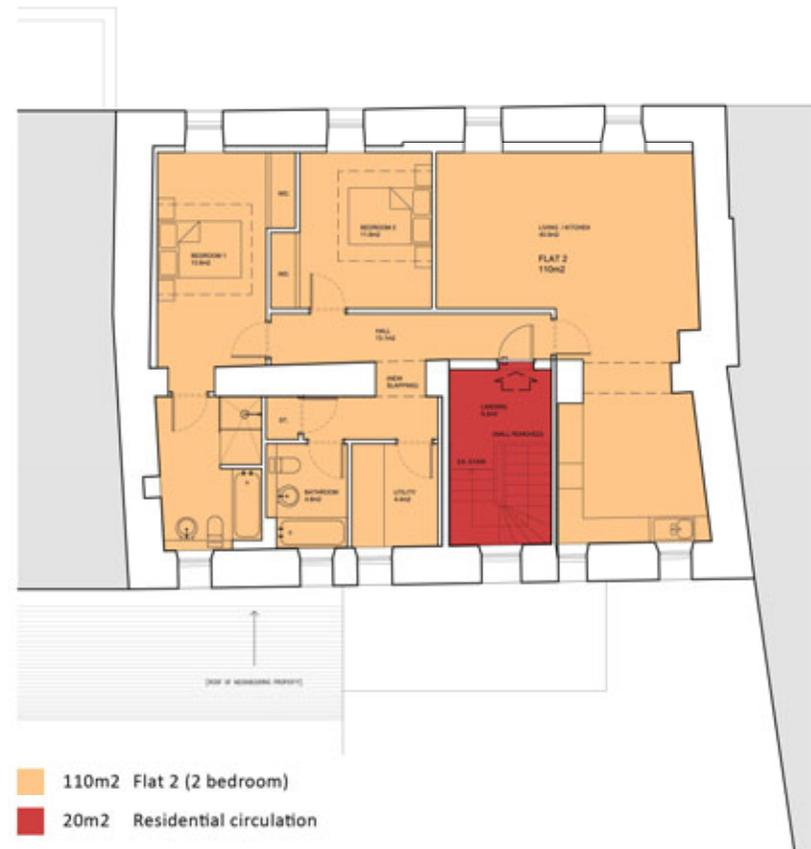
Figure 16: Second floor plan – as proposed. 2 bedroom flat
