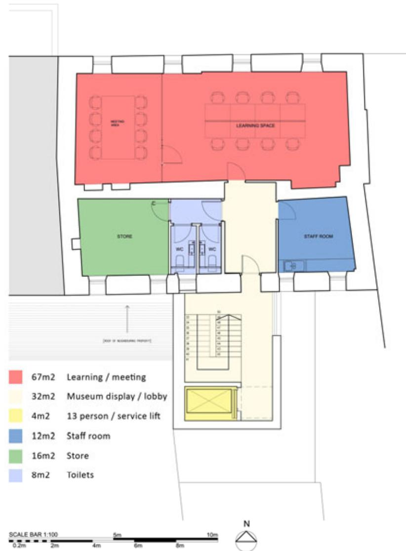
Figure 12: Second floor plan – Staff and archive area as proposed
