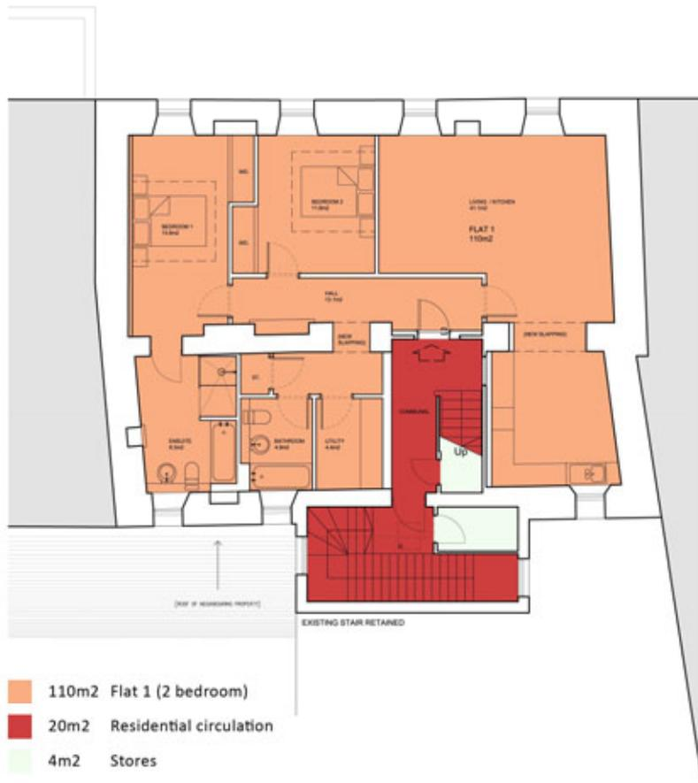
Figure 15: First floor plan – as proposed. 2 bedroom flat
