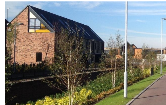
The Athletes Village in Glasgow included a strong green infrastructure framework from the outset. Swales are integrated into the streetscape to manage rainfall at surface. These green elements are designed to be safe and accessible meaning they did not require to be fenced off.
