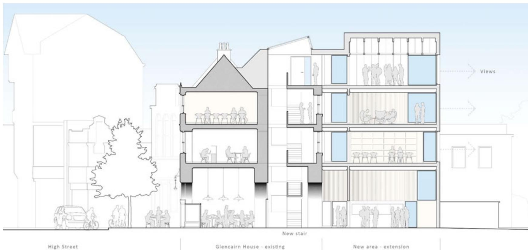
**Figure 17:** Development concept cross section
